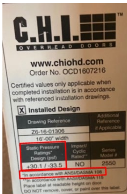
Figure 1. Photo of garage door label showing design pressure rating and test standard
